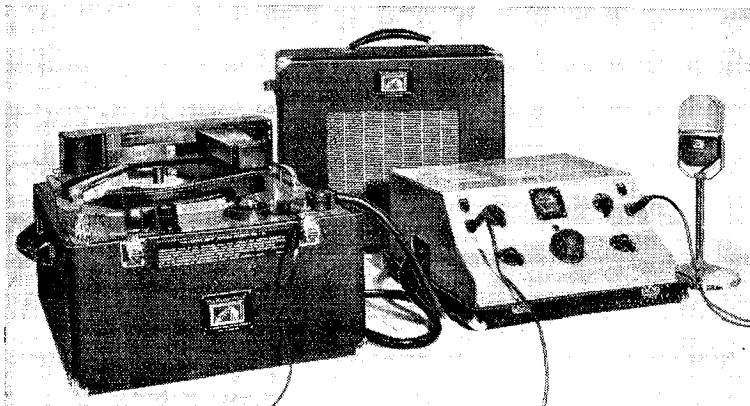
H.M.V. Model 2300H disc recorder. For transport, the equipment packs into three carrying cases.
